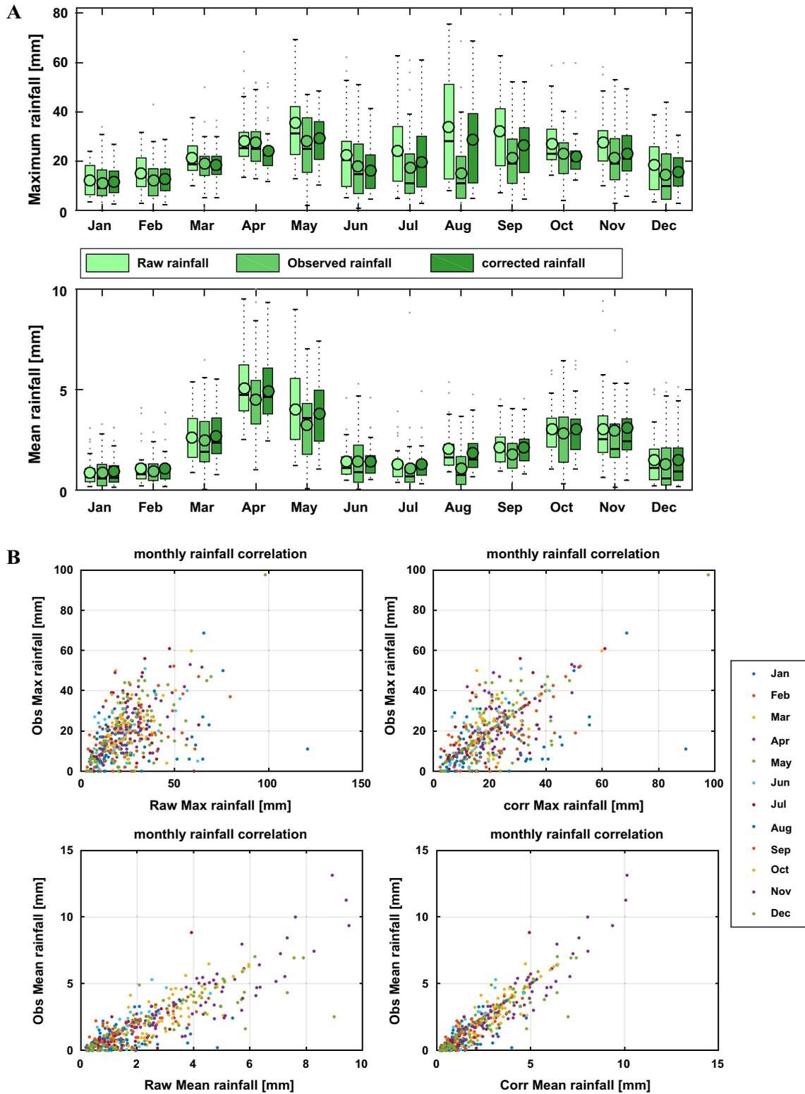
**Fig. 4** a Raw, observed and corrected maximum and mean precipitation at Dimika station. b Scatter plot of seasonal raw, observed, and corrected maximum and mean precipitation at Dimeka station
