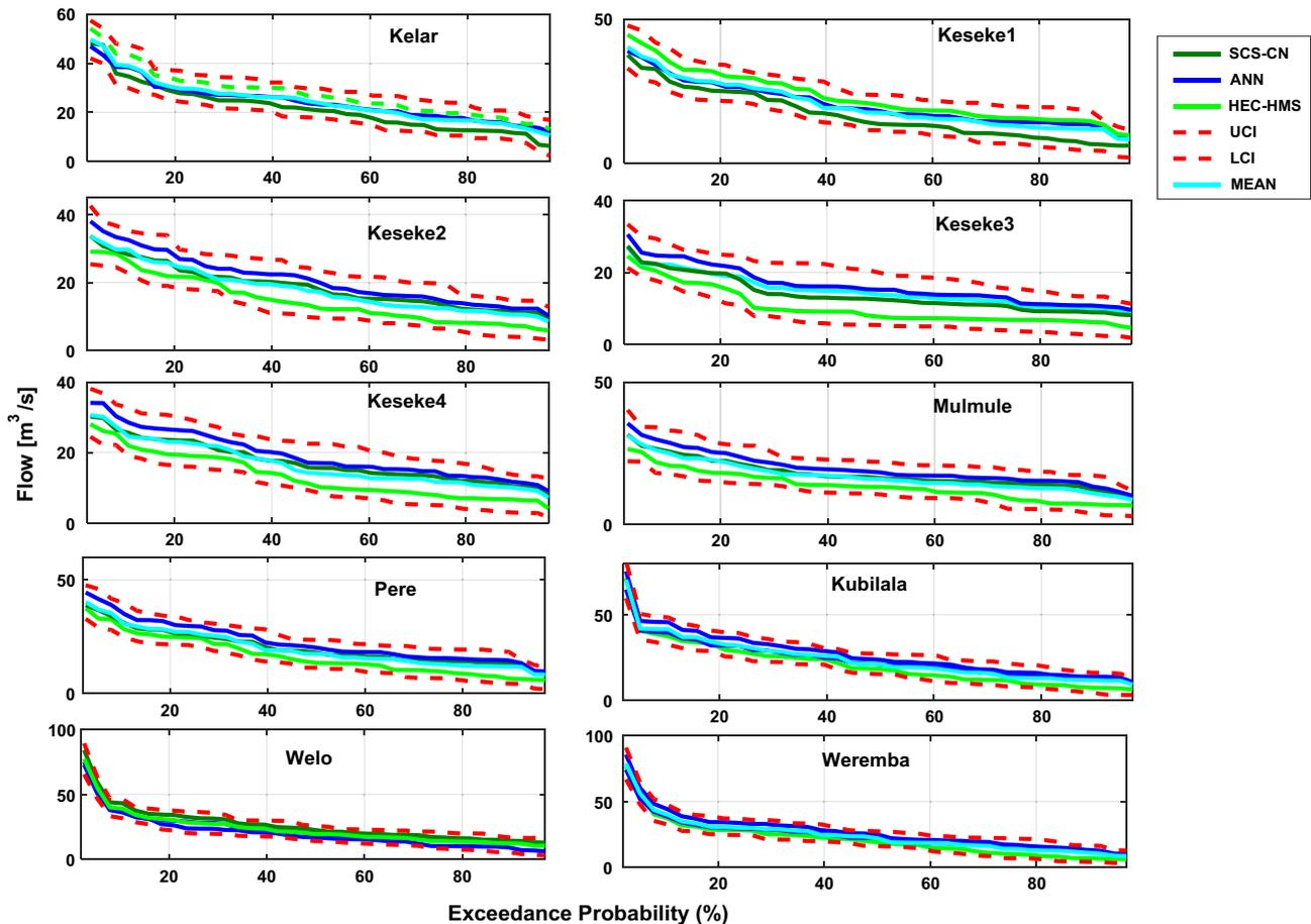
**Fig. 7** Exceedance probabilities of the estimated runoff using SCS-CN, ANN, HEC-HM and the 95% upper confidence interval, 5% lower confidence interval and mean at the selected stations
