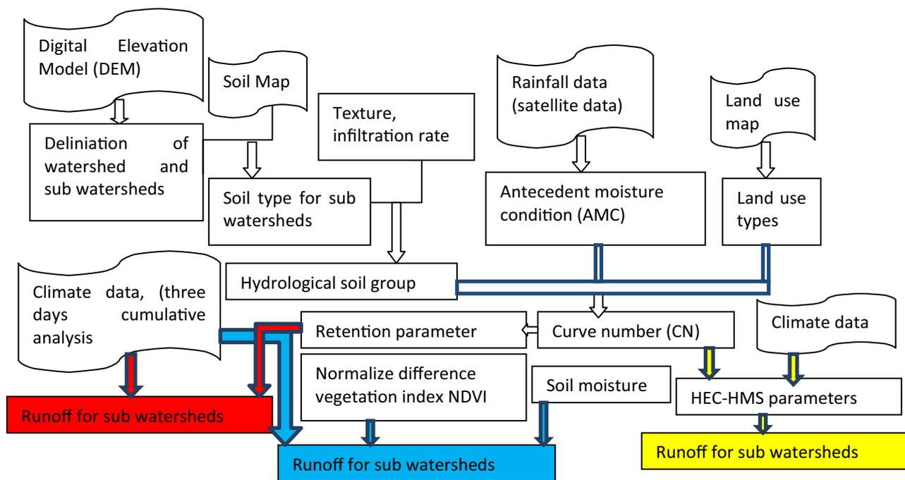
**Fig. 3** Methodological framework to estimate runoff value in ungauged catchment. Three river flow prediction techniques: (i) Red: empirical (SCS-CN), (ii) Yellow: hydrological model (HEC-HMS), and (iii) Blue: data driven committee model (ANN)
